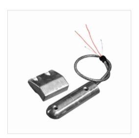
The Knight Fire & Security F10A is a Grade 2 roller shutter contact featuring a single reed switch, 4-wire connection, and 500mm armoured sleeving for enhanced cable protection. Designed for outdoor sheltered environments, this durable aluminium contact offers a 50mm operating gap, making it ideal for commercial and industrial security applications. Key Features:
